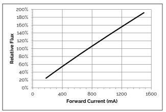
Figure 6: Flux vs. Current (1120mm only)
