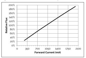
Figure 6: Flux vs. Current (1120mm only)
