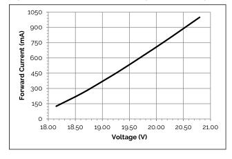
Figure 1: Current vs. Forward Voltage (280mm only)
