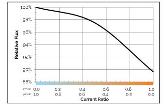
Figure 9: Flux vs. Current Ratio (2700K-6500K)
