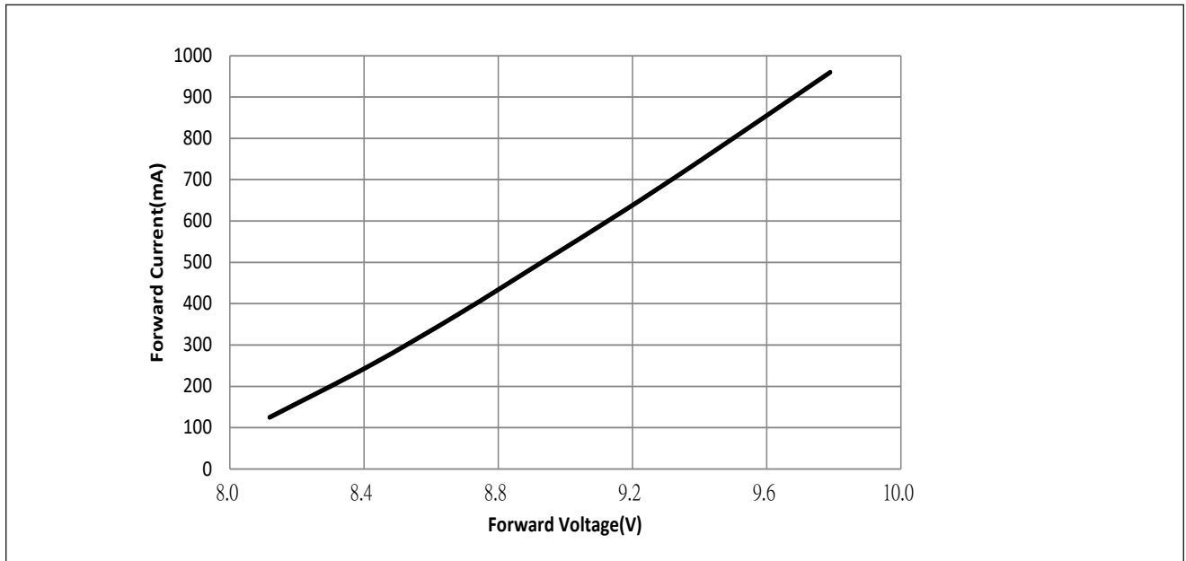
Figure 2: Drive Current vs. Voltage ( T_{sp}=25^{\circ}\text{C} )
