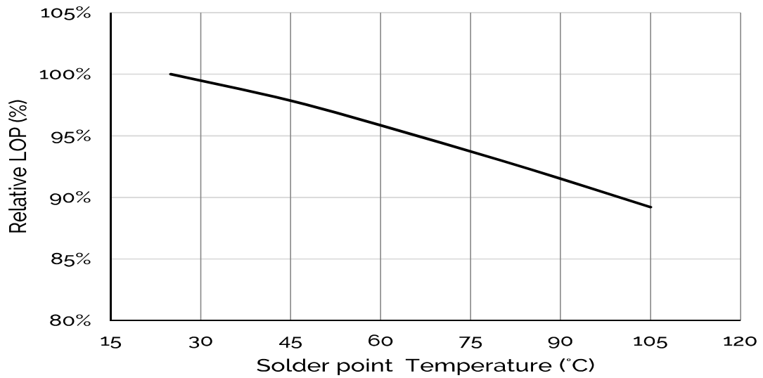
Figure 4: Typical Relative Flux vs. Solder Point Temperature
