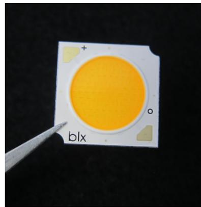
If pick-and-place equipment is used for automated assembly, the vacuum collet should be designed to avoid contact with the yellow phosphor resin area and the thin white ring surrounding the yellow phosphor resin area. Contact with the outer perimeter area of the array is acceptable.
