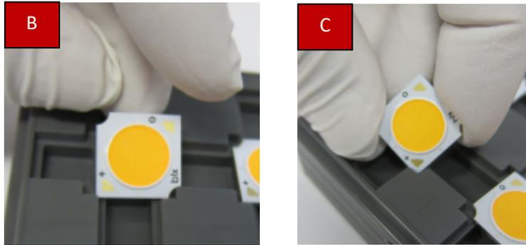
Figure 4: LED Arrays removal from the tray: (a) remove tray cover, (b) use a finger to push the array up away from its pocket, and (c) grip the arrays from the sides to lift the array out of the pocket while the arrays pivots on one corner
