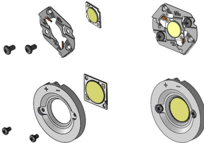
Figure 14: LED Arrays Holder Examples
