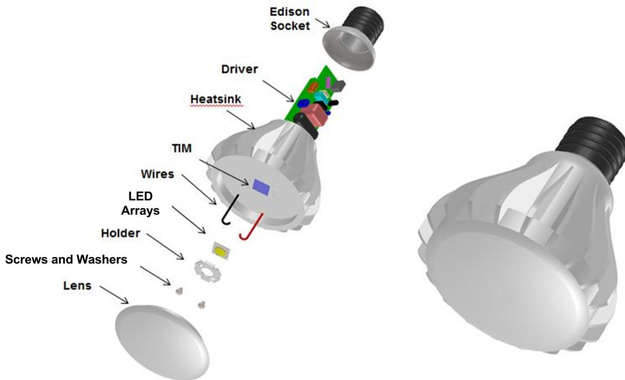
Figure 1: LED Array System Assembly Drawing
