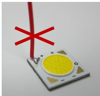
Figure 11: Example of problematic wire bending that induces stress on the solder joint
