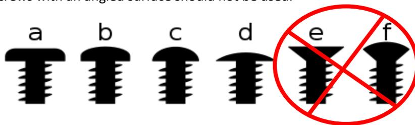
Figure 13: Screw Head Types for V Series
