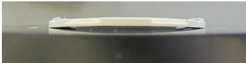
Figure 18: Typical Flex of LED Arrays Module
