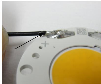
Figure 16c: Cold solder joint due to insufficient heat
