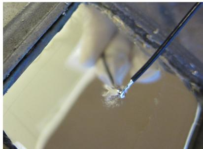
Figure 12b: Pre-tin the wire by dipping the tip of the wire in a solder pot
