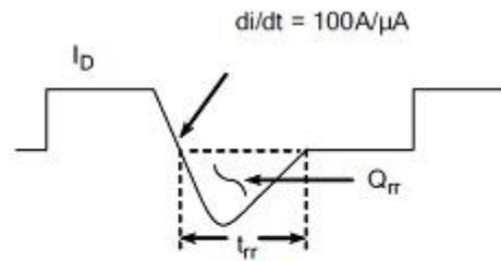
Diode Reverse Recovery Waveform
