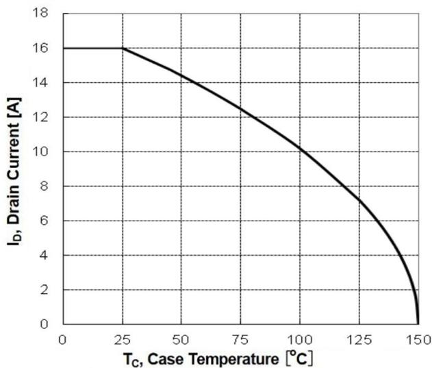
**Figure 10. Maximum Continuous Drain Current vs Case Temperature**
