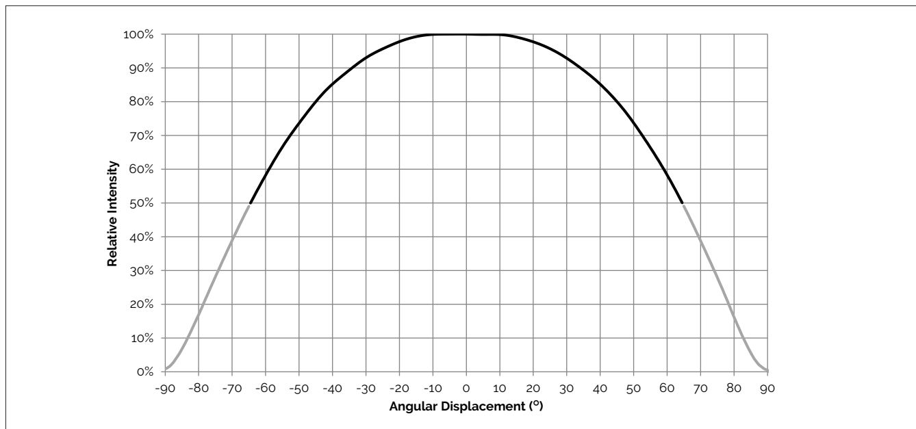
Figure 10: Typical Spatial Radiation Pattern
