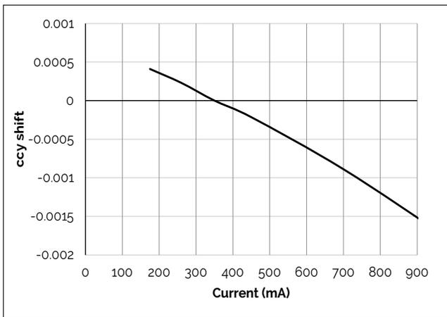
**Figure 10: Vero13C Drive Current vs. ccx Shift**
