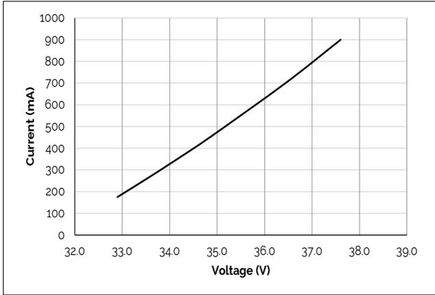
**Figure 2: Ver013C Drive Current vs. Voltage**
