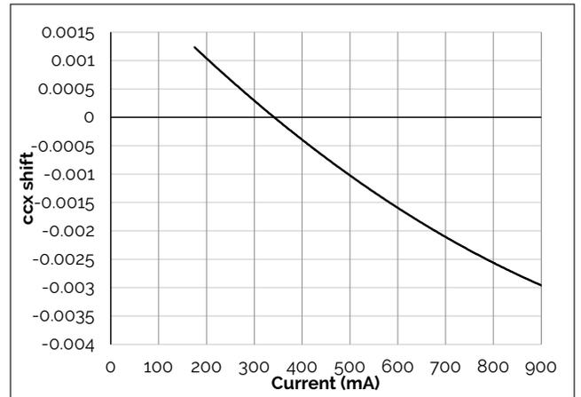
**Figure 9: Vero13B Drive Current vs. ccx Shift**
