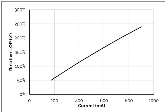
**Figure 4: Ver013C Typical Relative Flux vs. Current**
