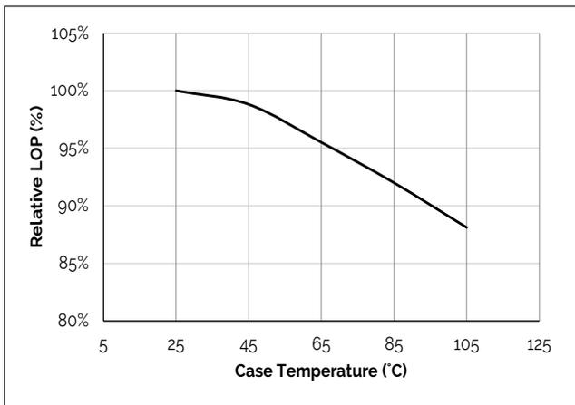
**Figure 6: Typical DC ccx Shift vs. Case Temperature**
