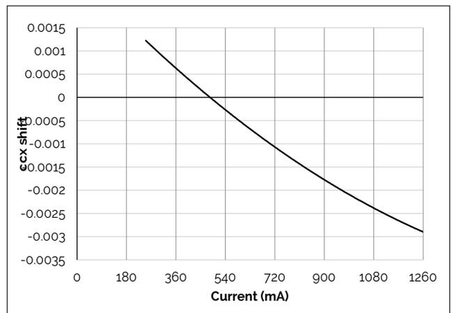
**Figure 11: Vero13C Drive Current vs. ccx Shift**
