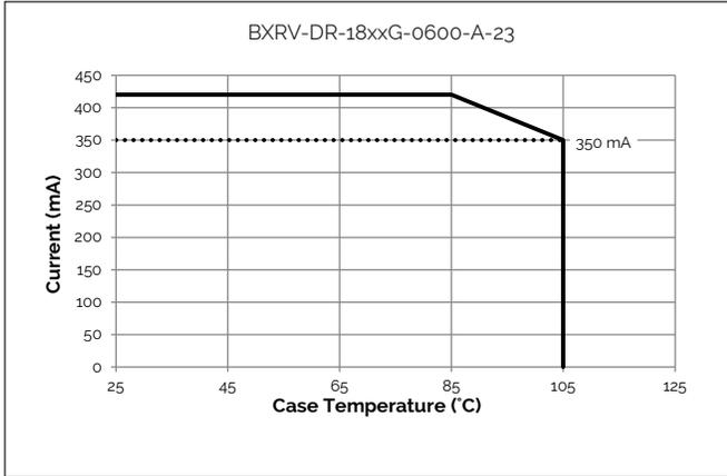
**Figure 12: Derating Curve**
