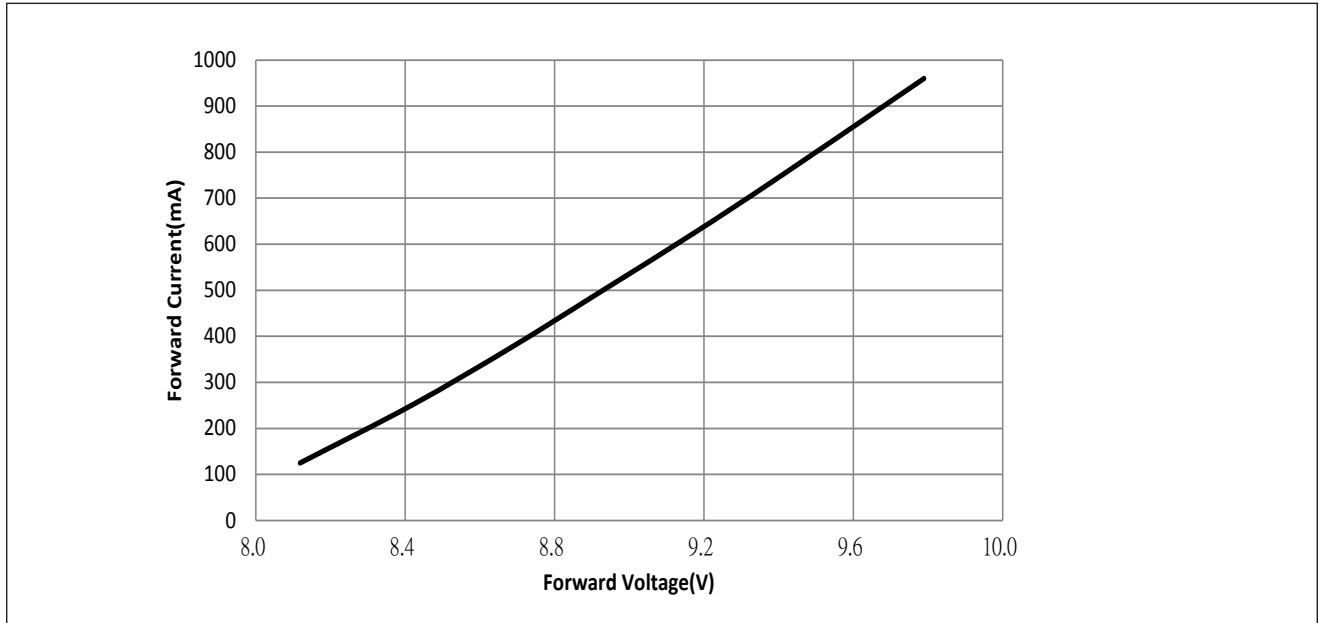
Figure 2: Drive Current vs. Voltage ( T_{sp}=25^{\circ}\text{C} )
