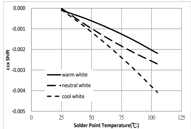
**Figure 7: Typical ccy Shift vs. Solder Point Temperature<sup>2,3,4,5</sup>**
