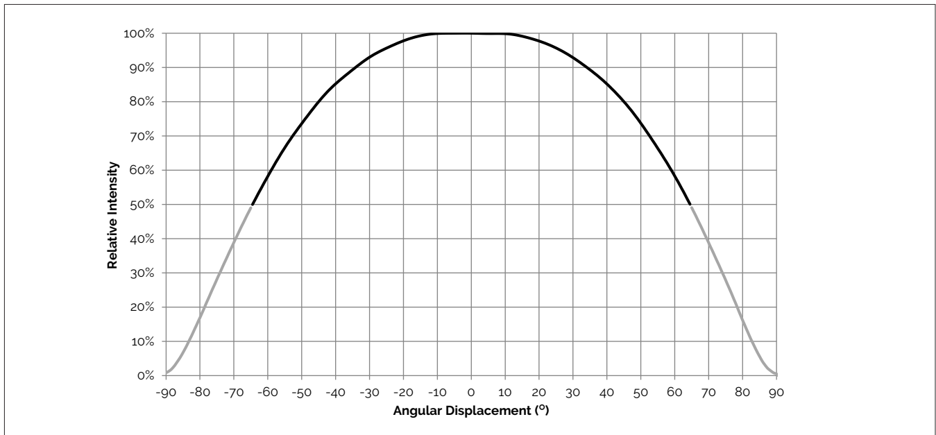
Figure 20: Typical Spatial Radiation Pattern
