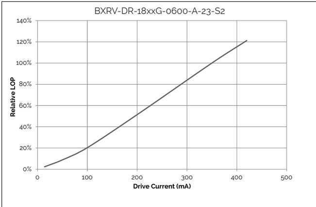
**Figure 6: Relative LOP vs. Drive Current,  $T_c = 25^\circ\text{C}$**
