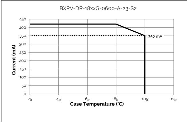
**Figure 12: Derating Curve**
