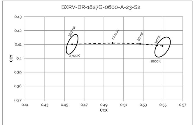
**Figure 15: Color shift vs. Forward Current 3000K - 1800K**
