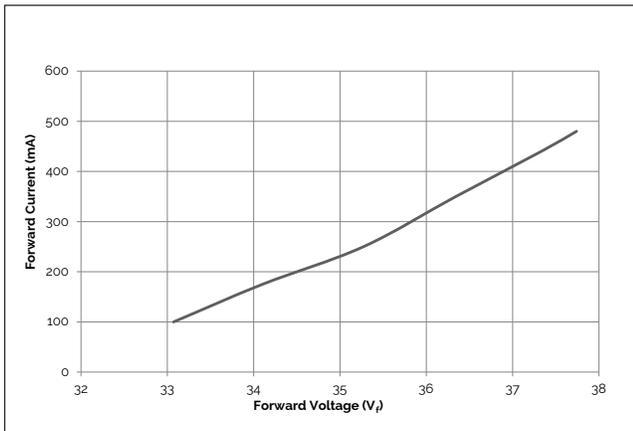
**Figure 12: Drive Current vs. Voltage V6G HD<sup>2</sup>**
