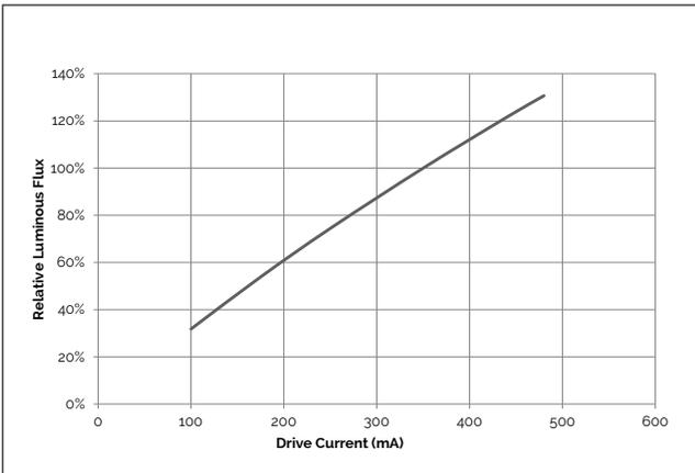
**Figure 14: Typical Relative Flux vs. Current V6G HD<sup>1,2</sup>**
