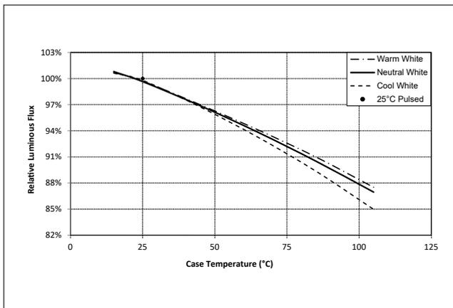
**Figure 16: Typical ccx Shift vs. Case Temperature**
