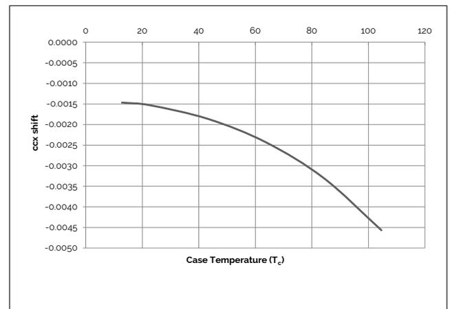
**Figure 17: Typical ccy Shift vs. Case Temperature**
